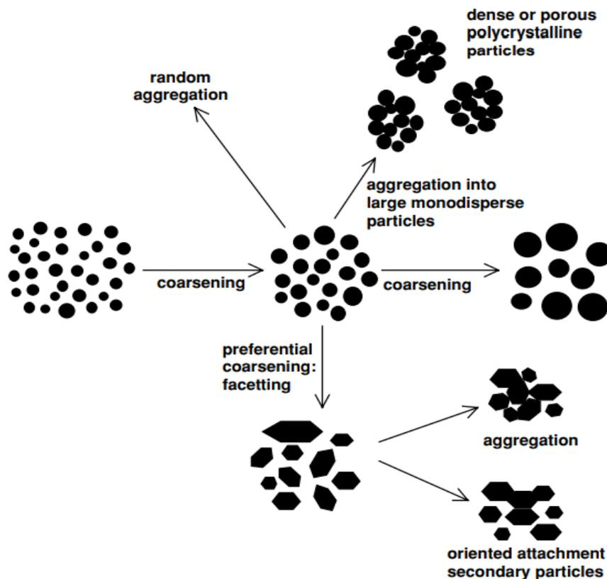
Figure 1: Diagram described how the shape of nanoparticles changing [10]
